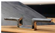
BITTE , rifiniture in acciaio e rivestimento in teak. CLEATS, steel finishing and teak flooring.
